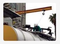
the loads generated by a cable type multi-span horizontal lifeline system. In addition, rigid systems eliminate sag and deflection, reducing the overall fall clearance needed below the work area.
