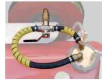
Decompression via the fire hose
