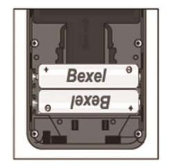
Note: do not charge rechargeable batteries in the breathalyser. Always remove rechargeable batteries and charge in a separate charger.
