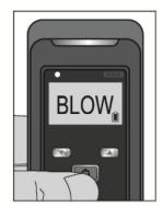
When the word BLOW appears, blow into the mouthpiece with a strong consistent breath. A beep will sounds while air is being accepted.
