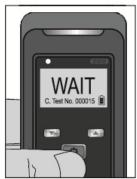
The word WAIT will appear on the display along with the number of tests performed since the last calibration
