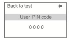
Note: If FAST MODE is set in the main menu (see pg. 12) press the down arrow when BLOW appears on the display and you can enter the User PIN Code entry screen.
