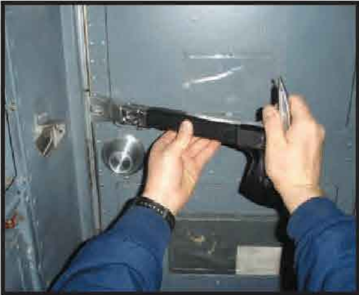
The Buster Tool is also used as a cockpit crash axe and exceeds (SAE) Aerospace Standard (AS) 5402 which specifies the design and performance criteria for aircraft crash axes.
