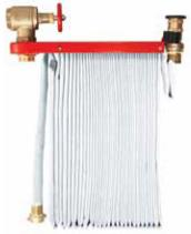
SRI's hose rack assembly is located inside buildings at the wet or dry riser outlet. It features a rack in which hangs the layflat fire hose (30m). An automatic release mechanism allows water to flow through the hose after removal of the hose and nozzle. The rack is available in sizes of 1-1/2" and 2-1/2". There are two methods of mounting the hose rack. One is by using a wall bracket and the other is by fixing on to a right angle valve.
