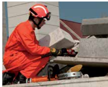
A perfect combination: crushing concrete with the CC 20 C and cutting re-bar with mini cutter CU 4007 C (or SMC 4006 C).
