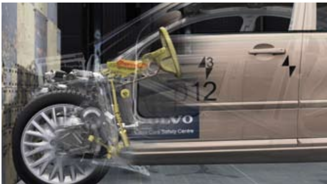
Crumple zone activated on impact. (A)
