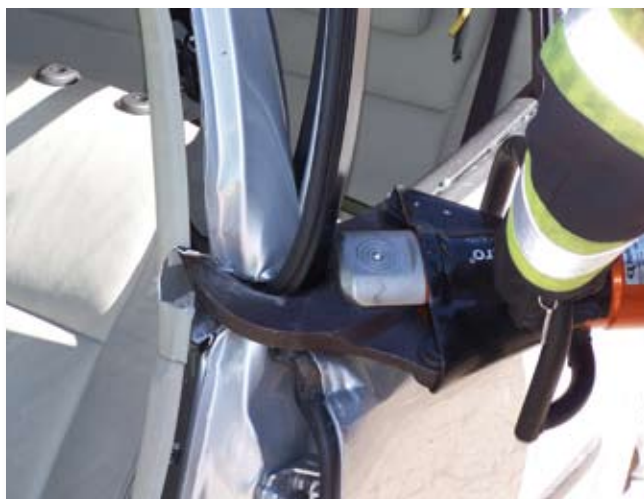
High-strength materials are pulled into the cutting recess to be cut at the strongest point of the cutter.
