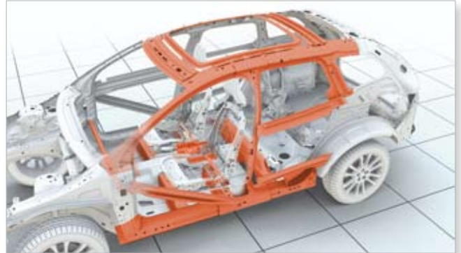
Passenger cell protected by reinforced construction. (D)
