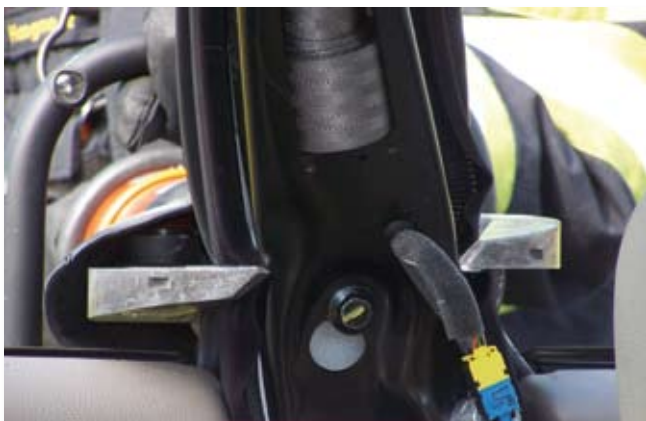
Holmatro's New Car Technology cutters are designed to surround and cut the wide, deep and reinforced pillars of the latest car models.
