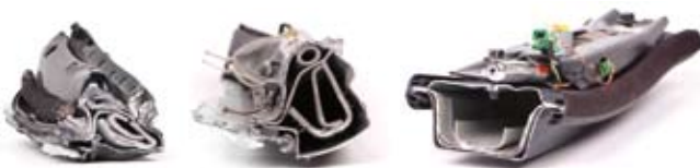
More examples of new and strong pillar constructions.
