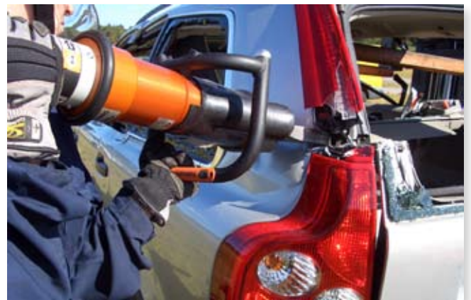
NCT™ II cutters also perform penetrating cuts with ease.
