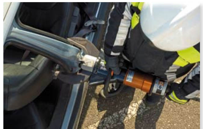
Holmatro's New Car Technology cutters are designed to surround and cut the wide, deep and reinforced pillars of the latest car models.
