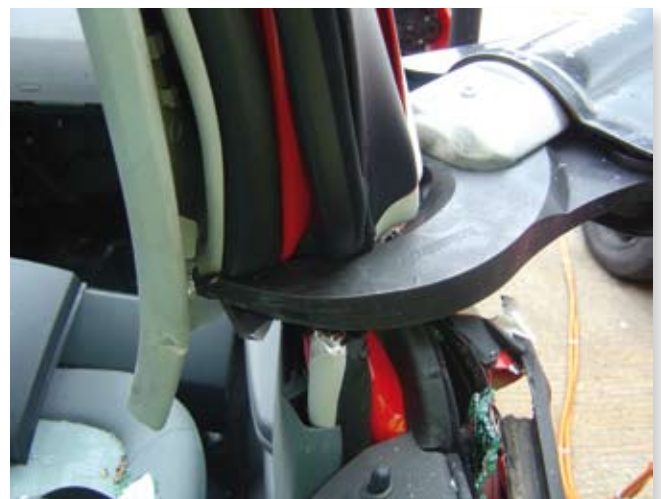
High-strength materials are pulled into the cutting recess to be cut at the strongest point of the cutter.
