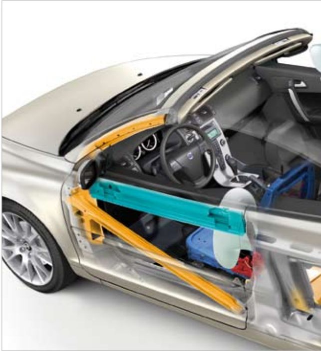
Door reinforcement to protect against side impacts. (E)
