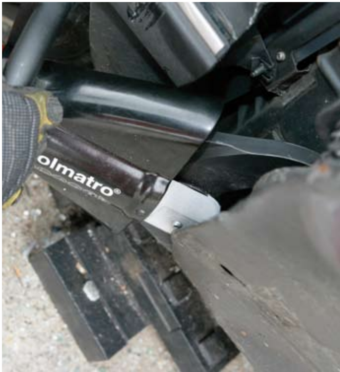
Better access to narrow spaces thanks to flat i-Bolt design.
