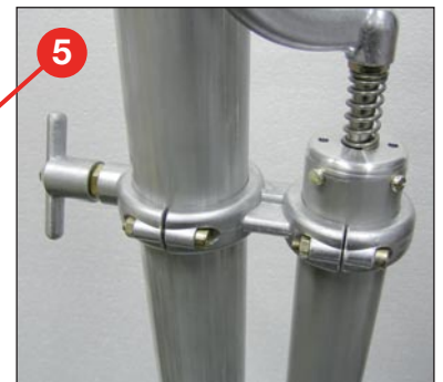
Handpump and clamp handle for quick and easy fitting onto a tripod or vehicle mounting bracket
