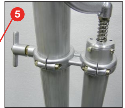
Handpump with top stud for quick and easy fitting onto a tripod
